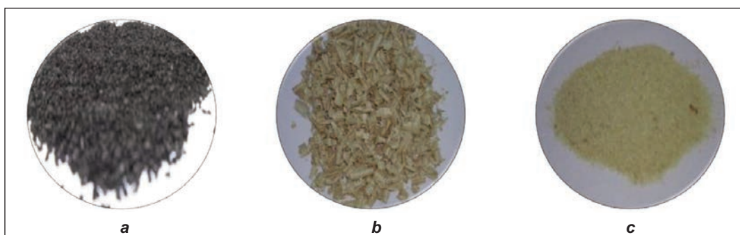
Fig. 2. Adsorbent materials: a – activated carbon; b – olive barks slices; c – olive barks powder after preparation
