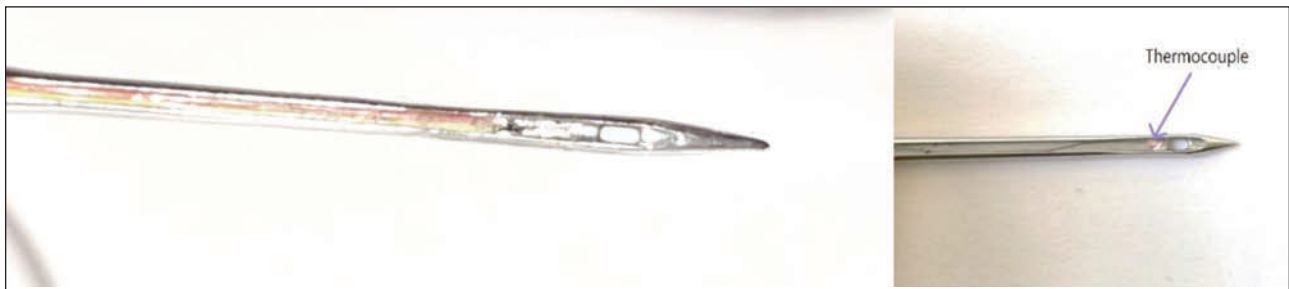
Fig. 3. The thermocouple is attached by soldering and welding techniques
