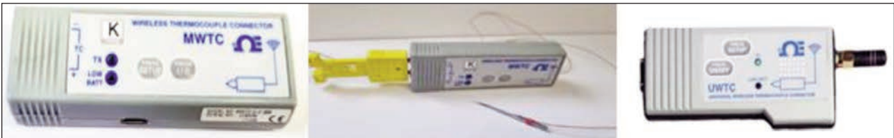
Fig. 6. Data logger and wireless connection device for K and C type thermocouple
